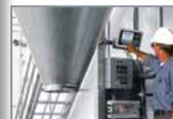
A 32-channel display capability allows viewing of weight on an individual scale and a combination of totaled scales.
