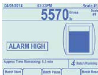
Bar graphs and visual cues inform users when a batch or fill is in process and when it's approaching target weights.
